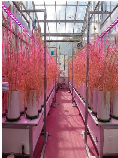
**FIGURE 1:** Wheat DroughtSpotter experiment shortly before grain harvest. Each pot contains one wheat plant and is placed on a dedicated weighing cell and watered by a dedicated spout. An environmental sensor (visible at left) records temperature, humidity and light within the greenhouse.
